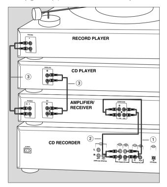
1 Connect supplied audio cable between the ANALOG OUT-sockets on the CD recorder and the ANALOG input sockets of the amplifier/receiver (TAPE, CD-R, AUX or PLAY IN, LINE IN).
